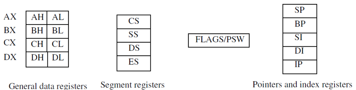
Fig.1.4 Register organization of 8086 Microprocessor
